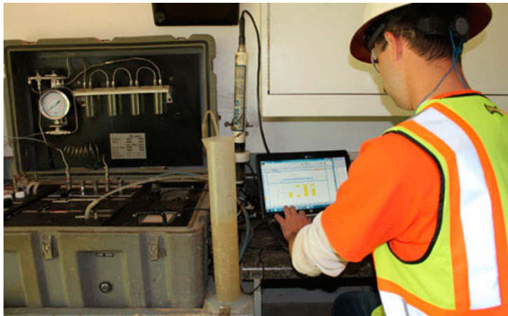
APS Groundwater Sample Collection
