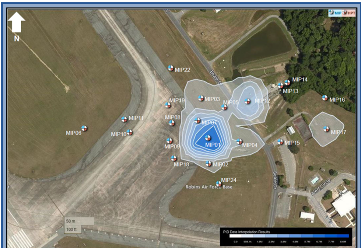
Contoured MIP photoionization detector (PID) data from the SSI at SWMU 57.
