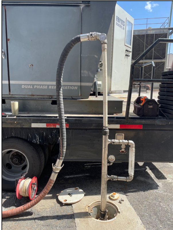
HVR unit well head stinger setup
