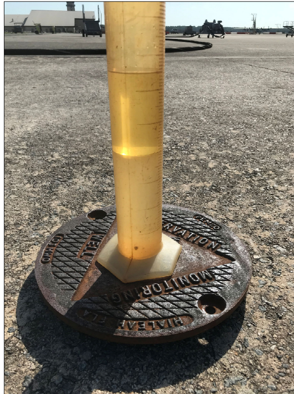
B45MW67 2-phase liquid, but both are clear
