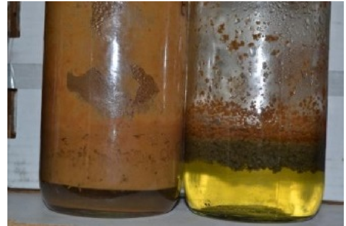
Photograph 1. Contaminated Groundwater Emulsion Before and After Treatment with De-emulsifier
