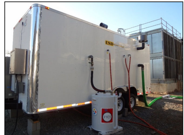
Remediation Trailer (↑) and LNAPL Collection Tank (↓)
