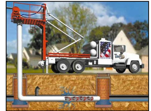
Slip lining utility pipe
