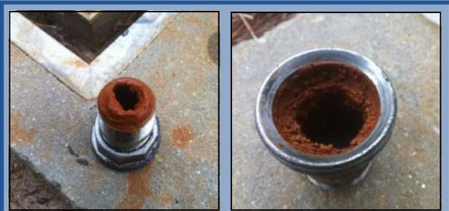
Iron deposition on extraction well caps at LF003.
