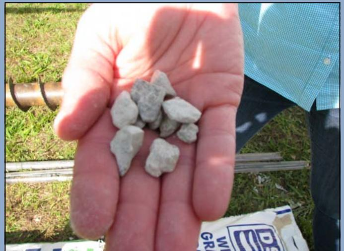
Close-up view of bentonite pellets used to seal annular space above the well screen.
