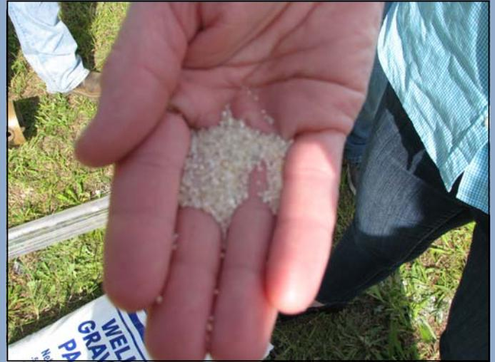
Close-up view of sand pack used between well screen and geologic formation.
