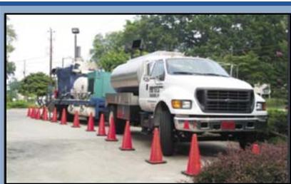
Example of a mobile multi-phase extraction system.
