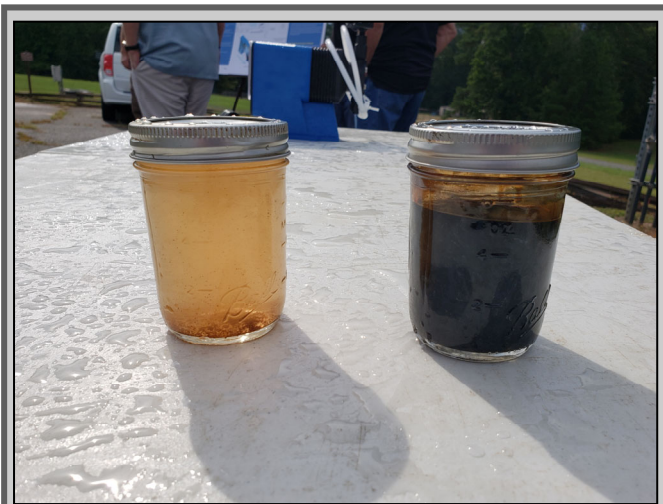
View of leachate from leachate collection wells (left) and NAPL from OWS (right).
