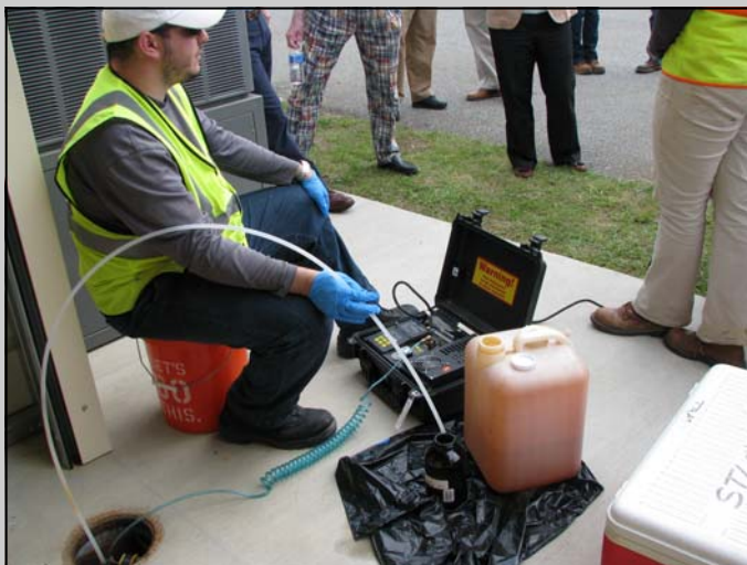
Collecting sample in amber bottle for analysis of semi-volatile organic compounds (SVOCs).
