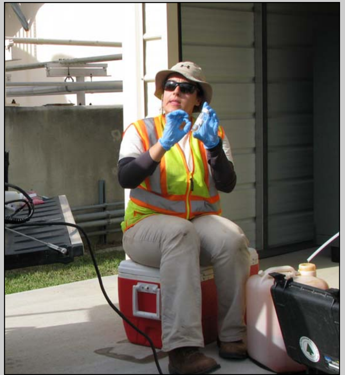
Collection of sample in 40-milliliter vials for analysis of Volatile Organic Compounds (VOCs).
