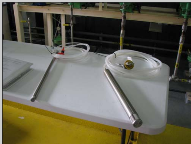
Close-up view of bladder pumps.
