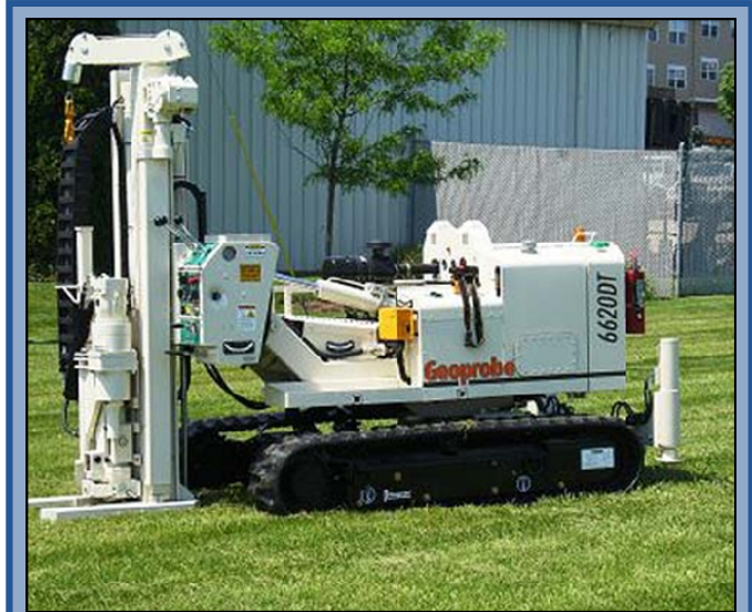
Example photograph of a DPT rig similar to the rig used for the soil borings at Building 169.
