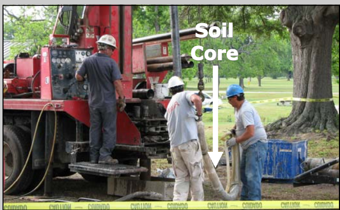
Representatives from Miller Drilling collect the four inch soil core from the core barrel in a plastic sleeve.
