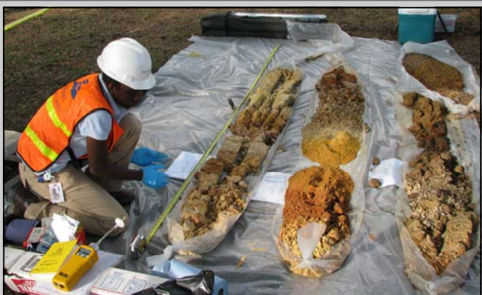
Dr. Lina Kodjo-Wayo, P.G., field geologist with Geosyntec, inspects the core to record the types of soil encountered during drilling.
