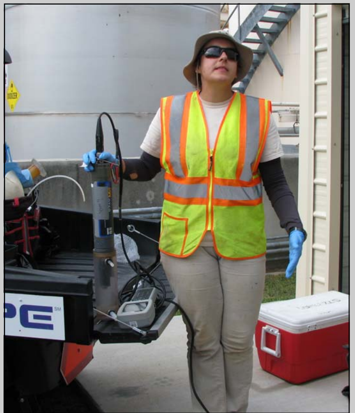
Water quality meter used to evaluate if groundwater quality has stabilized and groundwater sample can be collected.
