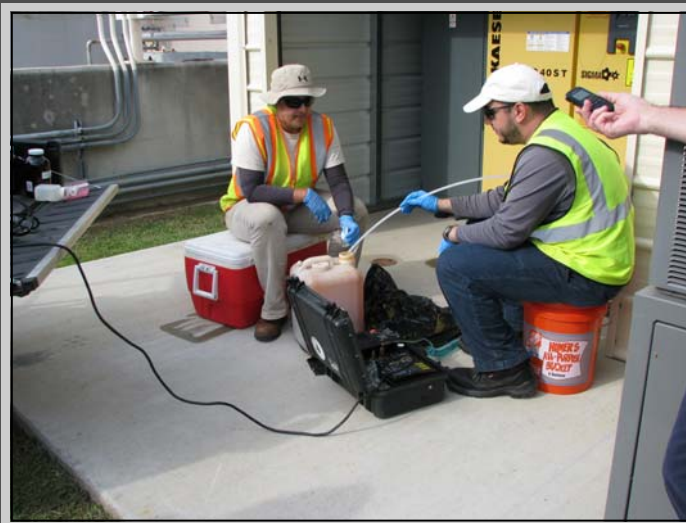
Collection of groundwater samples at LF1-4.
